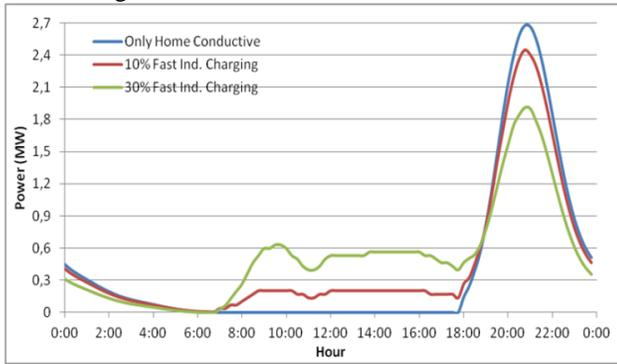
Fig. 6 EV demand in case 10% or 30% of the EV users rely on fast inductive charging solutions.
