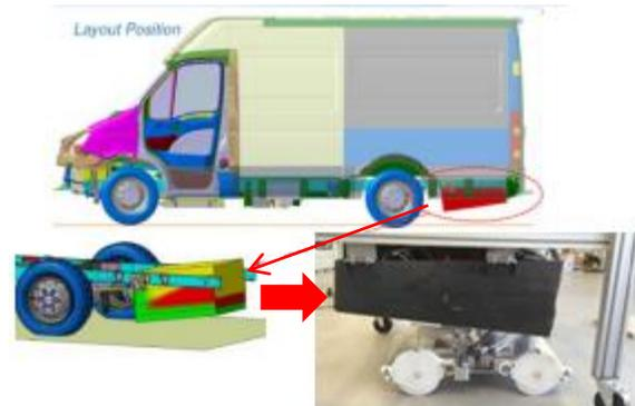
Fig. 3 Mechanical system aligning the gap between the primary and the secondary coil
