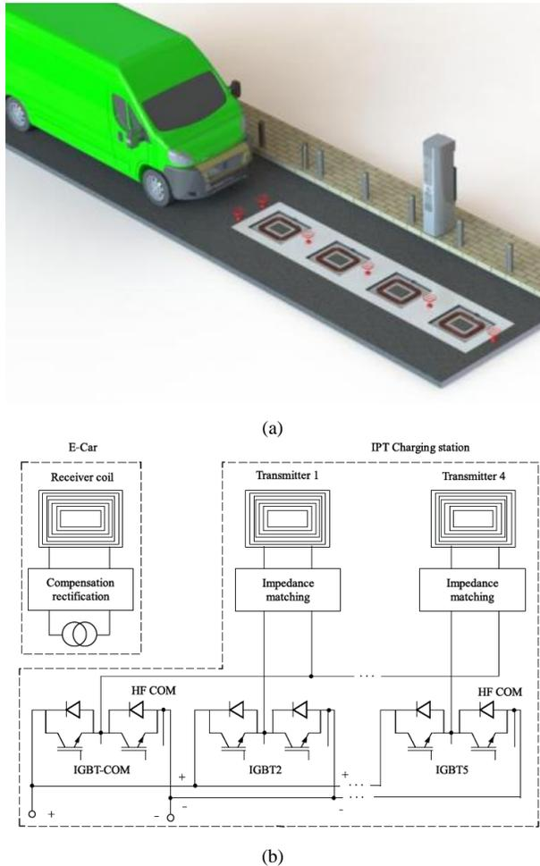
Fig. 4 (a) Implementation of the FastInCharge concept in an on-route application, (b) Power converter topology for an on-route inductive charging station [16]
