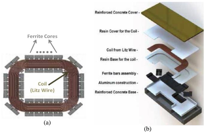
Fig. 2 (a) Design presented in the FastInCharge project, (b) 3D section view of the primary coil [14]
