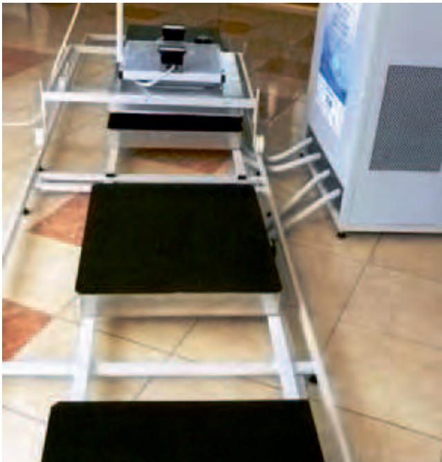
Fig. 5. Demonstration of the complete IPT system for static and on-route charging of EVs Converter 4 in 1, Transmitting coils (4 pcs), Receiver coil with rectifier and halogen indication, 30kW mm.
