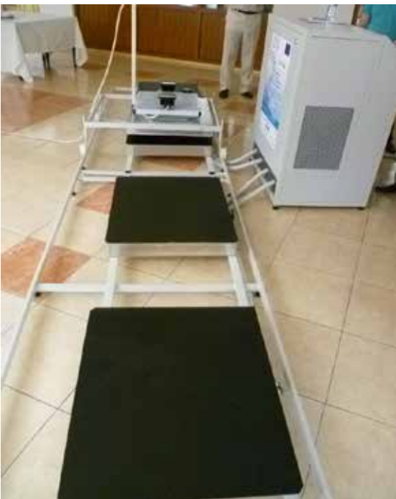
Figure 9. Demonstration of the complete IPT system for static and on-route charging of EV's - Converter unit, Transmitting coils (4 pcs), Receiver coil with rectifier and halogen lights indication
